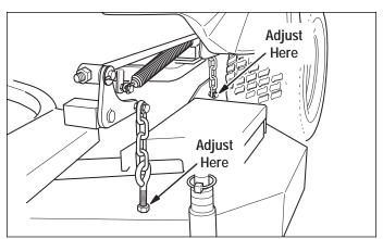
Figure 42. Deck Level Adjustment
